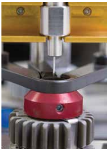
This autosampler can confirm the presence of certain taste-and-odor constituents detected by Metropolitan's Flavor Profile Panel.
